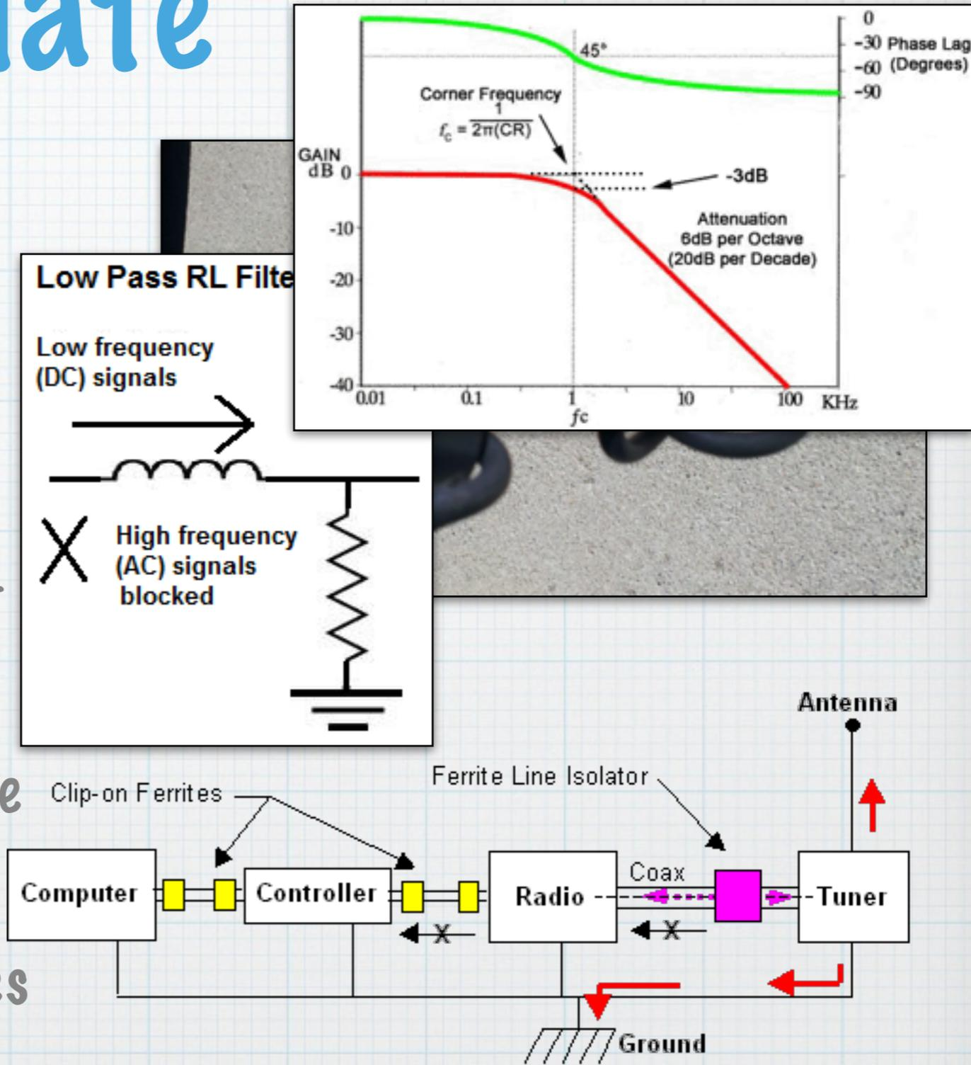
Fig 3: This is the same configuration as above with ferrite chokes added to block the alternative ground paths. Differential signal currents in the coax are not effected by the ferrite, but common-mode ground currents are blocked.
