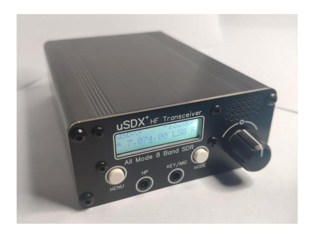
uSDR+ is optimized and modified based on the open source work uSDX/QCX-SSB uSDX/QCX-SSB GitHub:
