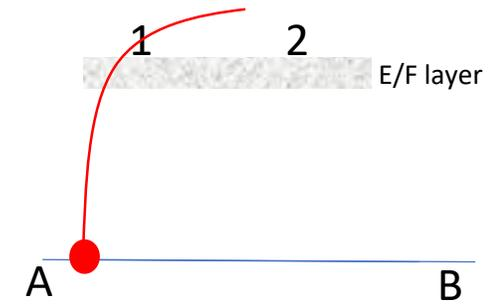
Paths that have refraction points inside or near the edge of the MUF isoline will hold propagation
