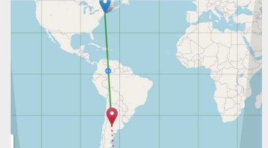
A to B path difficulty – North South, mid and low latitude paths are very reliable up to 28MHz even at the low of the sunspot cycle
