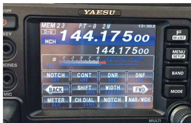
Figure 1 — The red portion of the ALC bar graph, extending beyond the blue bar operating range, indicates an excessive ALC setting.
